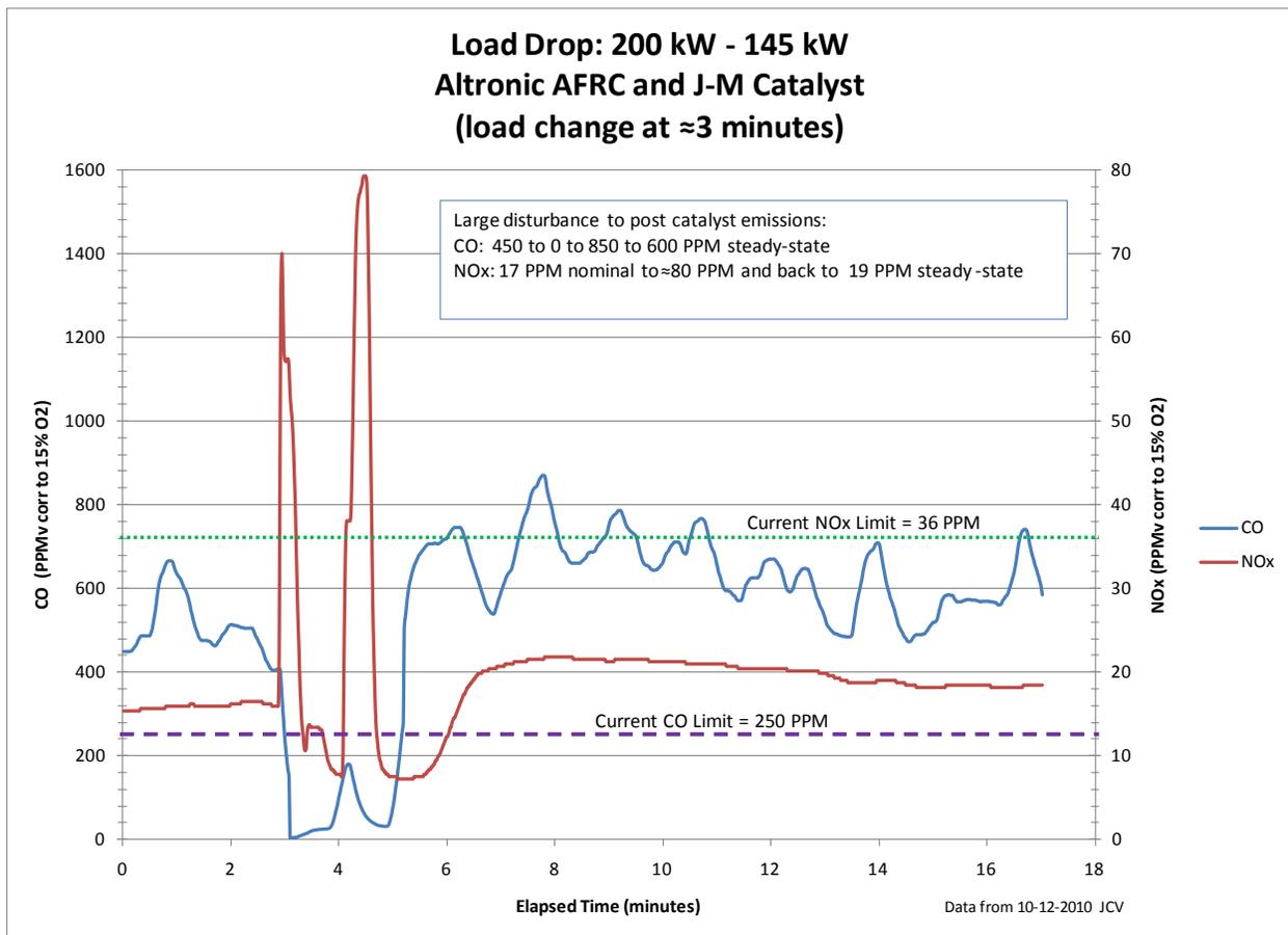
**Figure 16: Original Controller and Catalyst showing large upset to emissions from a load change**
