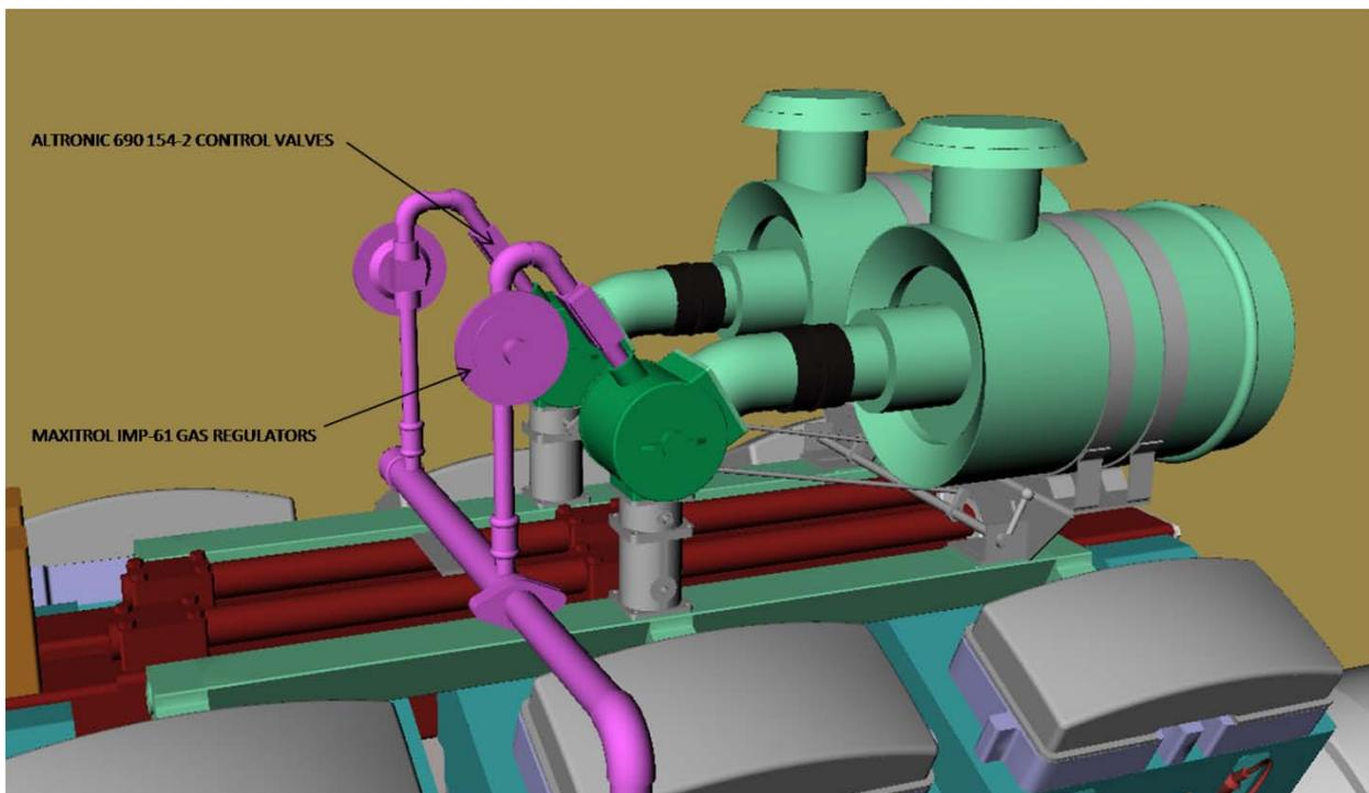
**Figure 5: Detail of components to be modified. The two small pressure regulators were re-used**
