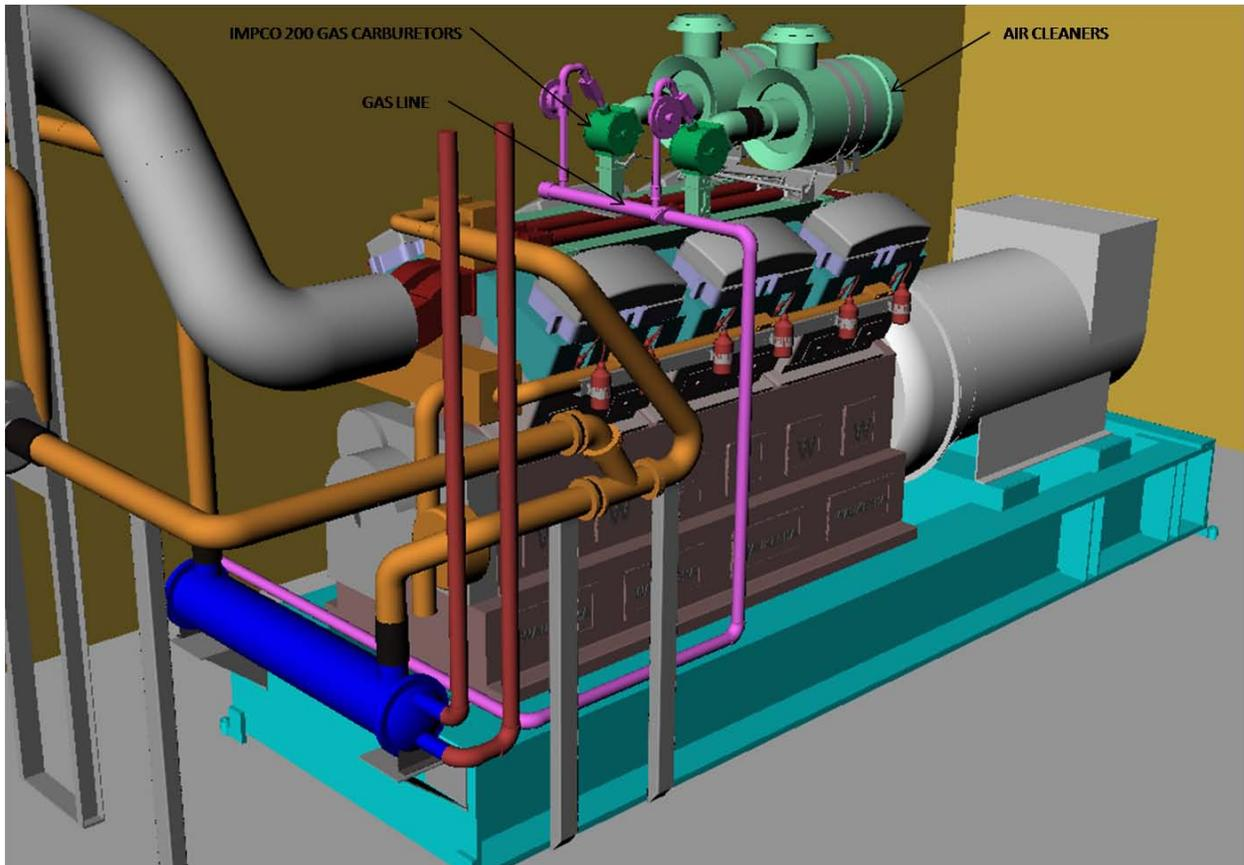
Figure 4: Solid Model of Engine Generated by the Project Team
