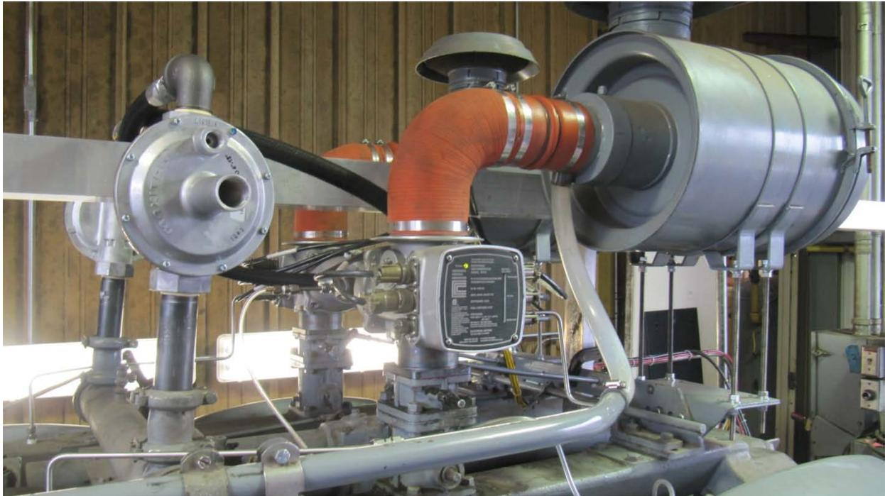
**Figure 12: View of reconfigured Fuel System and EGC4 installation.**
