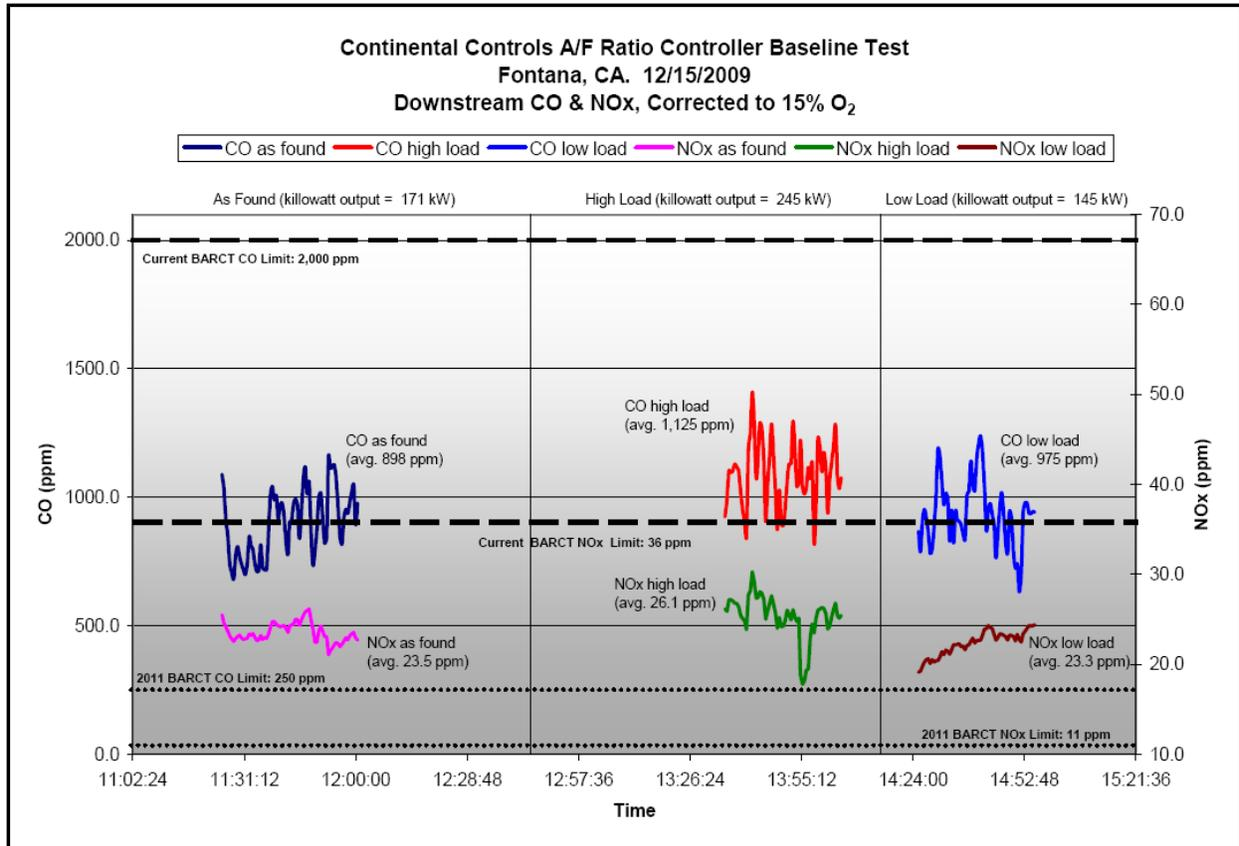
Figure 8 (above) and 9 (below): Baseline Emissions Data. Note fluctuations in the “steady-state data”
