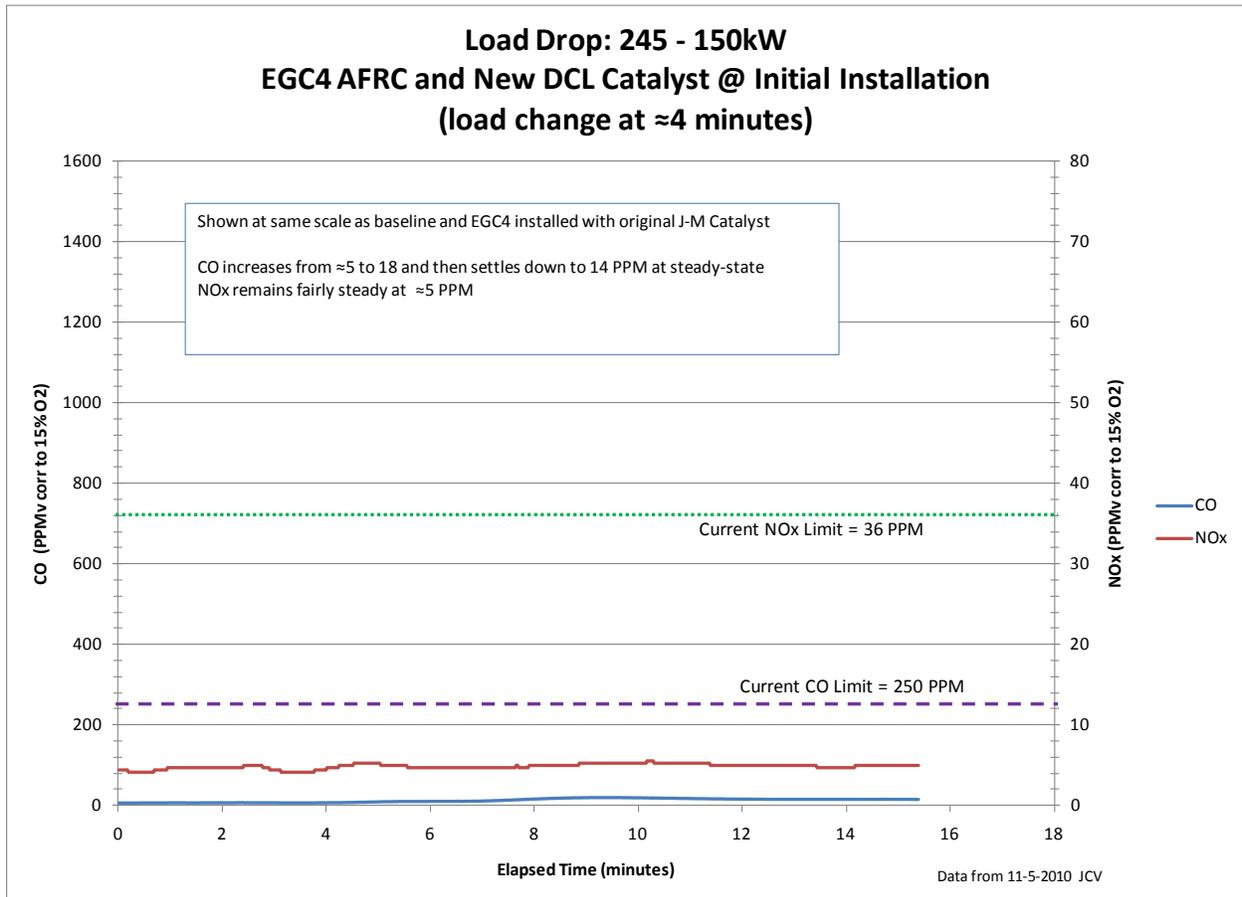
**Figure 18: New EGC4 Controller and New DCL Catalyst showing initial performance**
