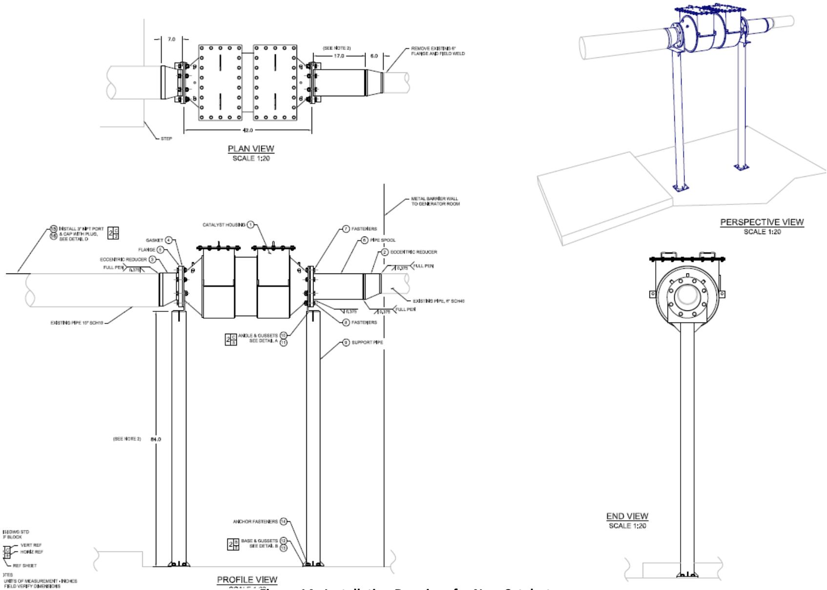
Figure 14: Installation Drawings for New Catalyst
